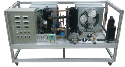
Multi compressor rack Ref. Trainer (AV-RH-R-7200)
