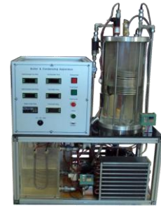
Steam Condensing System (AV-RH-A-1300GL)
